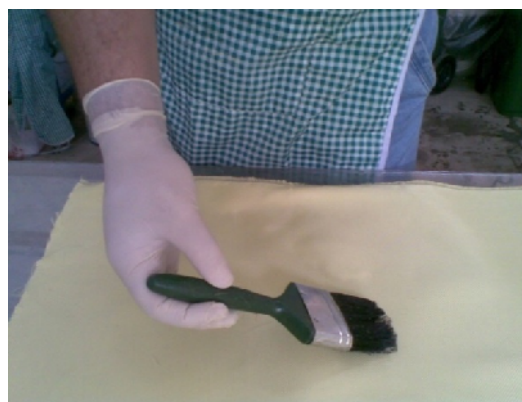
Fig 2: A Photograph show a Hand Lay-Up Process
